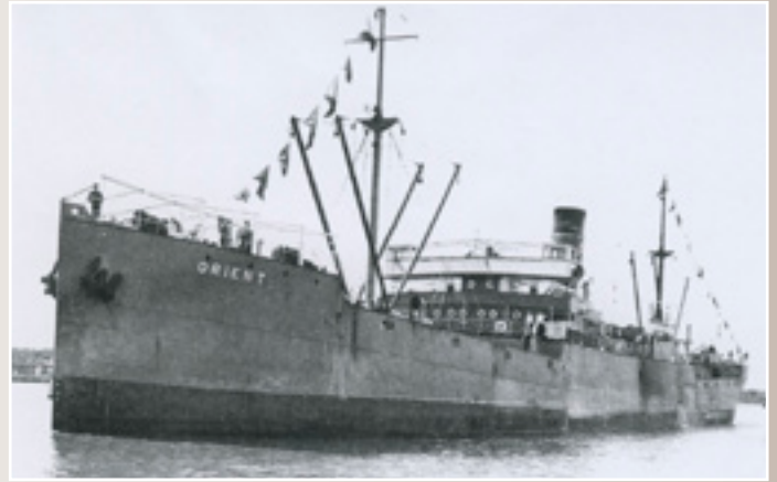
Ångfartygs Ab Bores/Orient Abs ss Orient, åren 1927–1934. 7600 dwt. Triple steam engine 3 cy. 2,625 IHP. (Foto: Oy Rettig Ab Bore)
